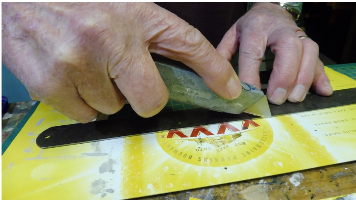
Above: Cutting the beer carton card using a Stanley knife and a steel rule as a guide. The cuts are done on a flexible cutting mat.
